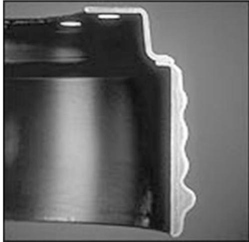
cast iron. The inner steel cage of brake drum is literally surrounded by cast iron providing excellent heat absorption throughout the drum while improving strength and drum life. The machined mounting face of the cast drum provides a solid supporting foundation for the wheels of the vehicle. This rigid mounting face assures a completely flat mating surface for positive wheel support.
