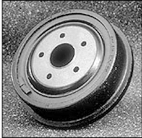
additional iron in the drum band and mounting areas in order to achieve the same strength. The steel drum back contributes to significant weight savings that result in increased payloads and improved fuel economy. The composite drum is developed out of a need to reduce the weight of passenger cars and light trucks.
