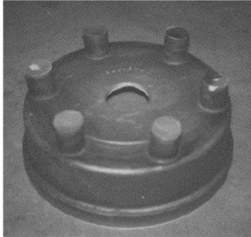
manufactured by dispersing coal fly ash in aluminium alloys. These composites offer cost saving low energy consumption and light weight. The Fig. 2.7 shows a fly ash reinforced MMC brake drum manufactured and studied in University of Wisconsin-Milwaukee. But the limitations are the segregation of low density fly ash composite, and mixing of this low density fly ash with the aluminium alloy.
