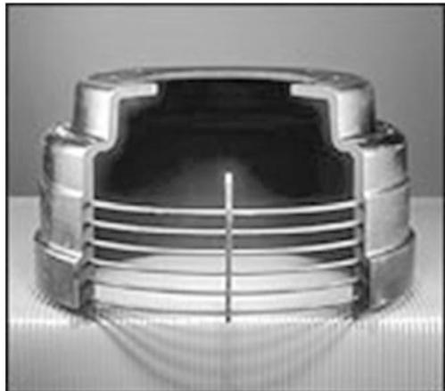
**Fig. 2.7** Fly ash reinforced brake drum
