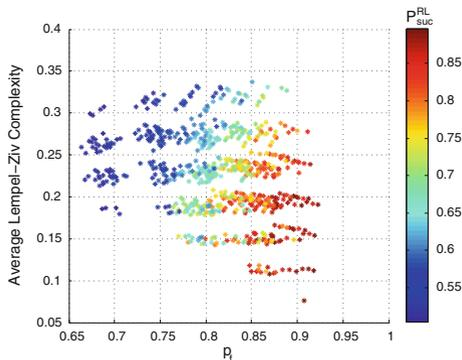
**Fig. 2.3** ISM band (indoor), TCD dataset. Probability of success of Q-learning as a function of the average LZ complexity and the probability of at least one free channel existing. Each point represents a particular instance of Q-learning applied to  $N = 3$  channels. The total number of possible combinations which we analyzed is  $\binom{17}{3} = 680$ , where 17 is the number of channels with  $DC \in [0.3, 0.8]$
