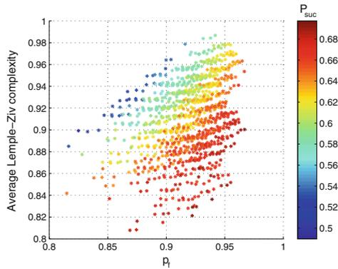
**Fig. 2.5** GSM1800 band (outdoor), RWTH Aachen dataset. Probability of success of Markov process-based learning algorithm as a function of the average LZ complexity and the probability of at least one free channel existing. Each point represents a particular instance of Markov process-based learning algorithm applied to  $N = 4$  channels. The total number of possible combinations which we analyzed is  $\binom{15}{4} = 1365$ , where 15 is the number of channels with  $DC \in [0.3, 0.8]$
