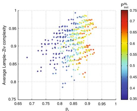
**Fig. 2.2** GSM1800 band (outdoor), RWTH Aachen dataset. Probability of success of Q-learning as a function of the average LZ complexity and the probability of at least one free channel existing. Each point represents a particular instance of Q-learning applied to  $N = 3$  channels. The total number of possible combinations which we analyzed is  $\binom{15}{3} = 455$ , where 15 is the number of channels with  $DC \in [0.3, 0.8]$
