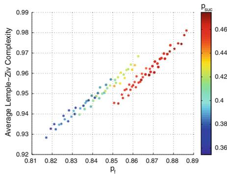
**Fig. 2.6** DECT band (indoor), RWTH Aachen dataset. Probability of success of Markov process-based learning algorithm as a function of the average LZ complexity and the probability of at least one free channel existing. Each point represents a particular instance of Markov process-based learning algorithm applied to  $N = 4$  channels. The total number of possible combinations which we analyzed is  $\binom{10}{4} = 210$ , where 10 is the number of channels with  $DC \in [0.3, 0.8]$
