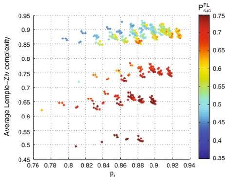
**Fig. 2.1** ISM band (outdoor), RWTH Aachen dataset. Probability of success of Q-learning as a function of the average LZ complexity and the probability of at least one free channel existing. Each point represents a particular instance of Q-learning applied to  $N = 3$  channels. The total number of possible combinations which we analyzed is  $\binom{15}{3} = 455$ , where 15 is the number of channels with  $DC \in [0.3, 0.8]$
