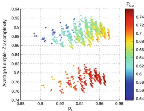
**Fig. 2.4** ISM band (outdoor), RWTH Aachen dataset. Probability of success of Markov process-based learning algorithm as a function of the average LZ complexity and the probability of at least one free channel existing. Each point represents a particular instance of the algorithm applied to  $N = 4$  channels. The total number of possible combinations which we analyzed is  $\binom{15}{4} = 1365$ , where 15 is the number of channels with  $DC \in [0.3, 0.8]$
