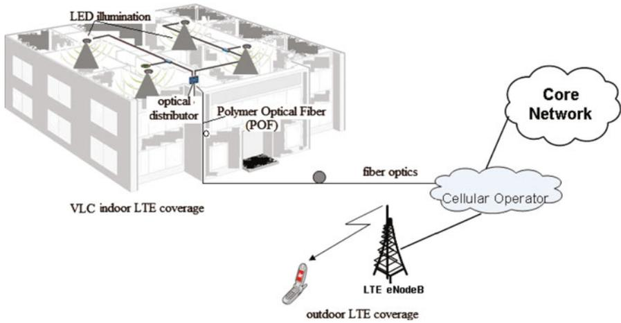
Fig. 2.2 VLC indoor LTE coverage implementation proposal
