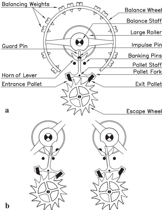
guide pin dips into a recess in the hub can the lever flip and let the escape wheel advance by half a tooth. This intermediate period of stalling the anchor allows the balance wheel to swing through angles as high as  $330^\circ$  to  $360^\circ$  with periods of typically 1/4 to 1 seconds (Fig. 3.14b). As a further innovation came pellets of low-friction metal inserted at the ends of the anchor.
