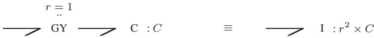
Fig. 2.22 Equivalence of an I energy store to a gyrator–C energy store combination
