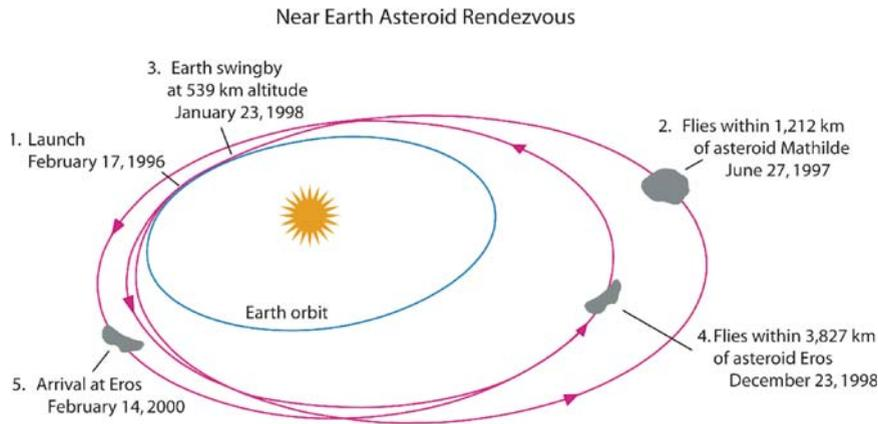
**Figure 2.12.** Trajectory of the NEAR spacecraft to 433 Eros. Courtesy of the Applied Physics Laboratory, Johns Hopkins University, and NASA.
