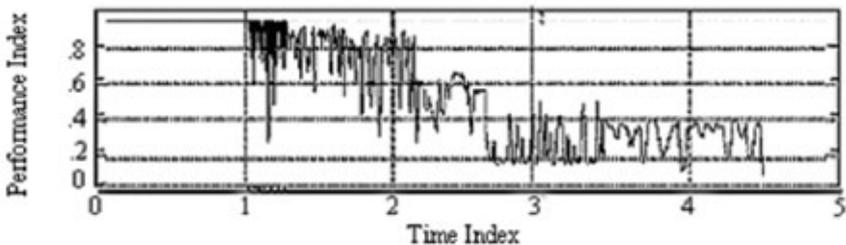
**Figure 2.21.** MV benchmark index for re-tuned MP separator (Loop 2)
