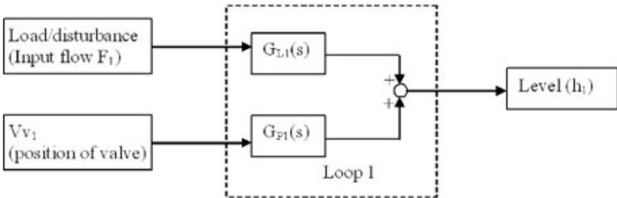
Figure 2.13. Block diagram for Loop 1: slugcatcher vessel
