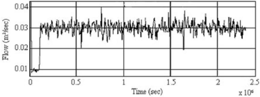
**Figure 2.26.** Crude oil output flow from MP separator
