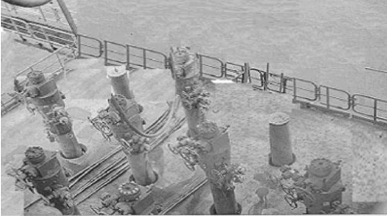
**Figure 2.4.** Production platform christmas tree and wellhead assembly
