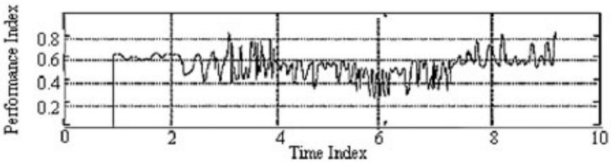
**Figure 2.19.** MV benchmark index for MP separator control (Loop 2)
