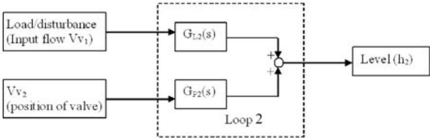
**Figure 2.14.** Block diagram for Loop 2: freewater knockout vessel
