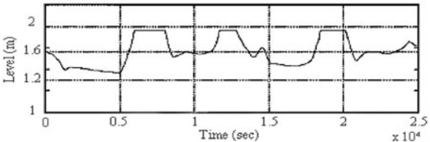
Figure 2.23. Re-tuned MP separator level (Loop 2)
