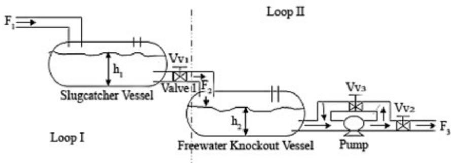
Figure 2.12. Schematic diagram for simplified 2 stage separation process
