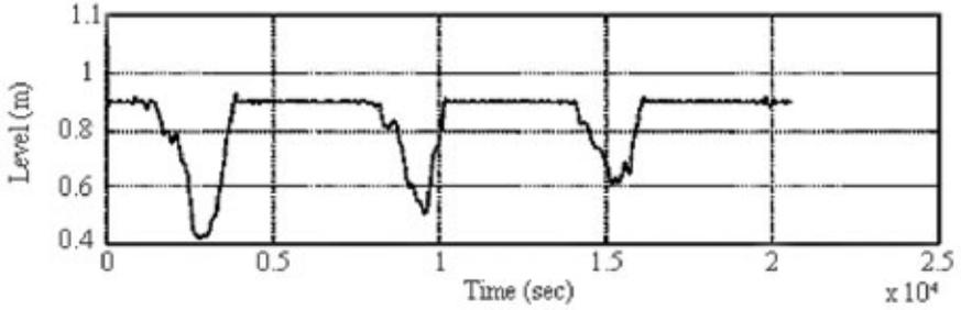
Figure 2.22. Re-tuned HP separator level (Loop 1)
