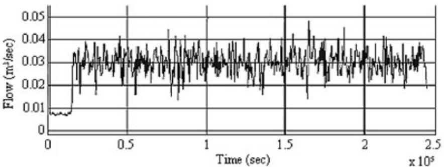
**Figure 2.25.** Crude oil output flow from HP separator
