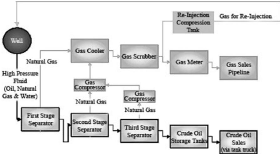
Figure 2.7. Gas compression and re-injection system
