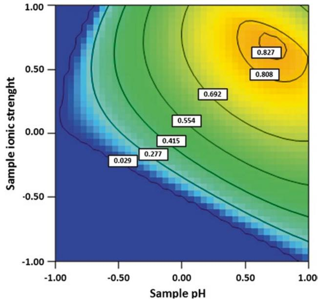
**Fig. 4** Contour plot exhibiting the interactive effects of sample ionic strength and sample pH while the sample load is maintained at 2.76 mS/cm. *Blue* areas correspond to combination of variables in which  $D=0$  (Color figure online)
