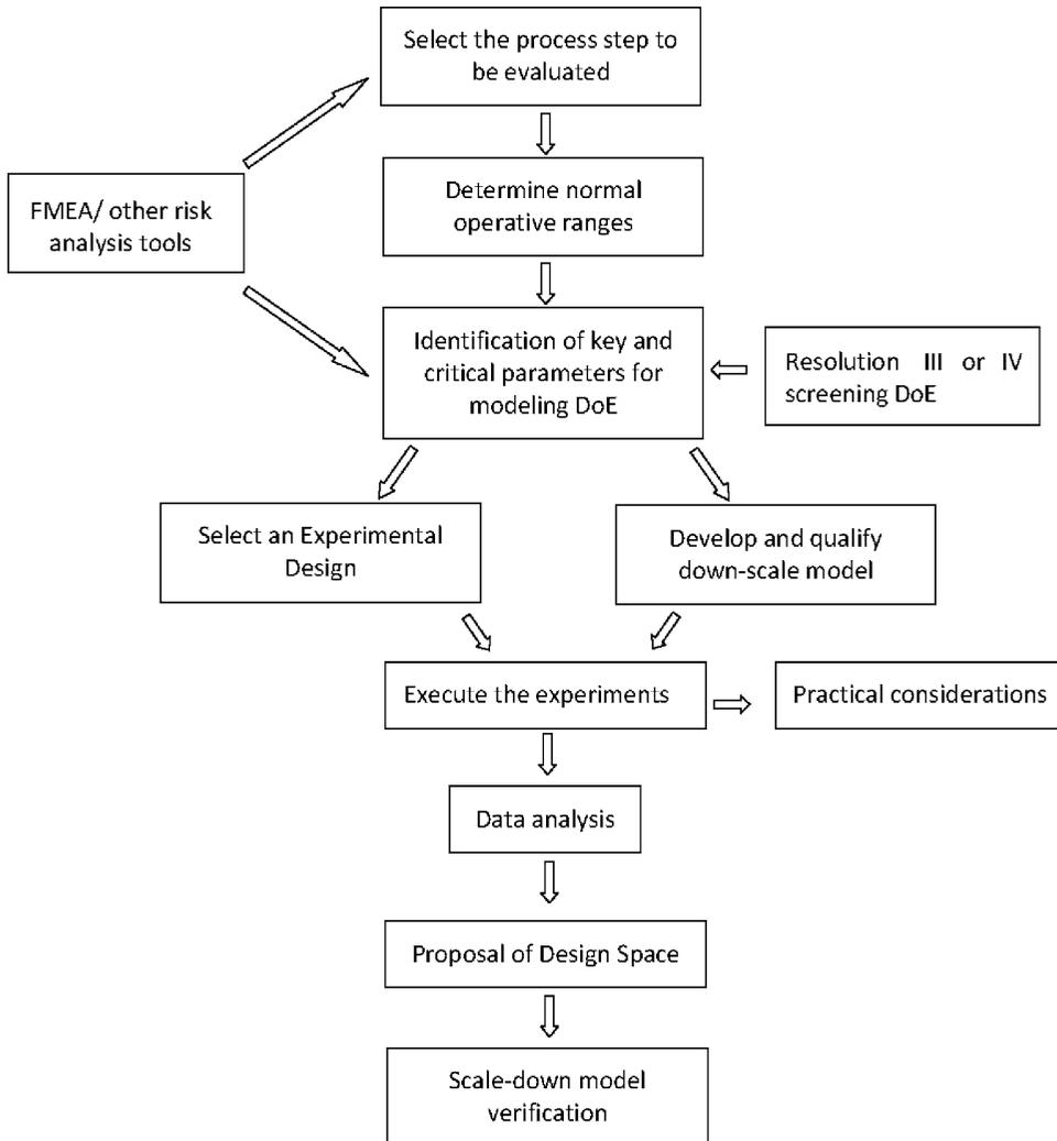
**Fig. 1** Sequence of activities toward the establishment of an expanded design space elements design space to applying DoE in a purification process
