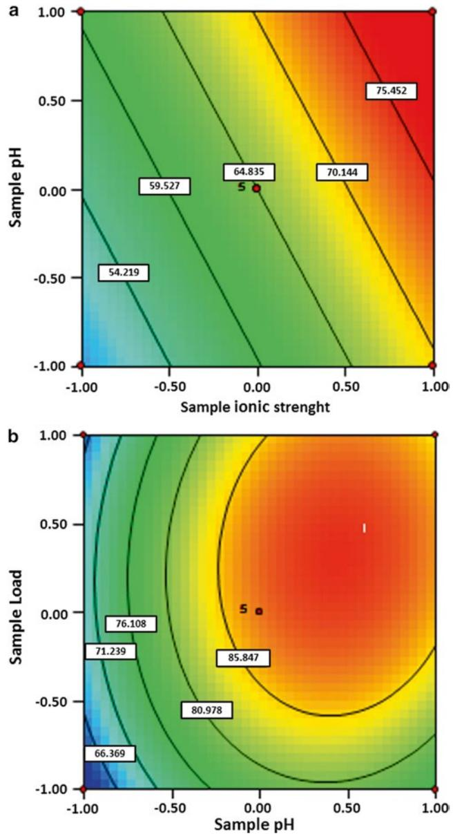
**Fig. 3** Contour plots showing the effect of the mutual interactions between two independent variables (the other variable is held at its center level) on every response. (a) sample pH and sample ionic strength effect on purity (b) sample load and sample pH effect on yield
