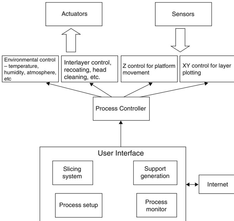
**Fig. 2.1** General integration of an AM machine
