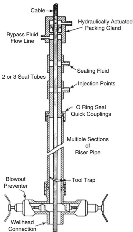
**Fig. 2.1** Production logging wellhead pressure-control assembly. Courtesy Schlumberger
