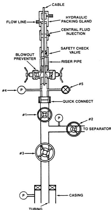
**Fig. 2.2** Correct Christmas-tree arrangement for production logging
