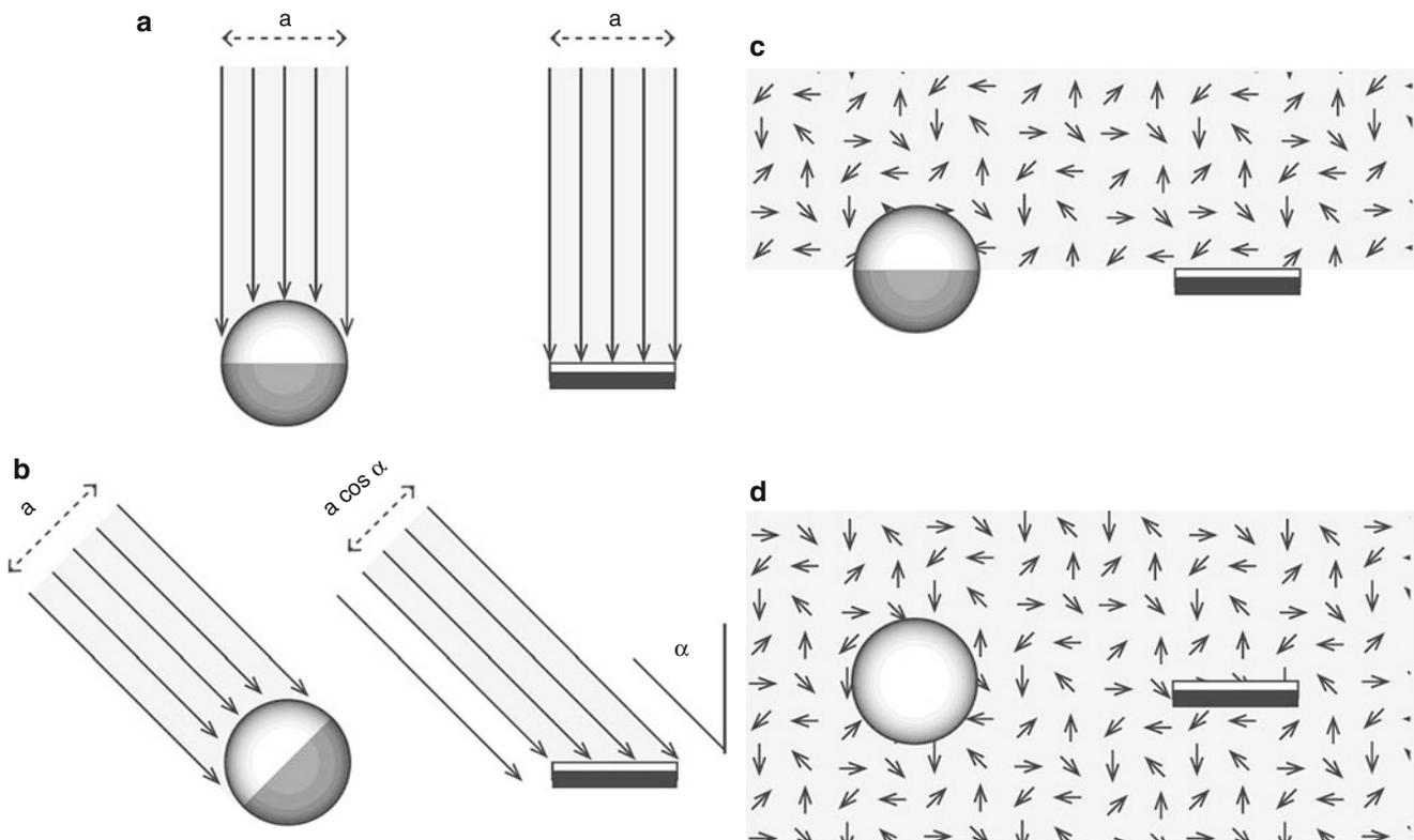
**Fig. 2.1** The concepts of irradiance and fluence rate. In (a) the incident light is perpendicular to the surface of the flat irradiance sensor. In this case, fluence rate and irradiance are equal. In (b) the incidence angle is  $\alpha$ . The irradiance sensor then intercepts only the fraction  $\cos \alpha$  of what the fluence rate sensor does. In (c) the light is diffuse, but incident only from
