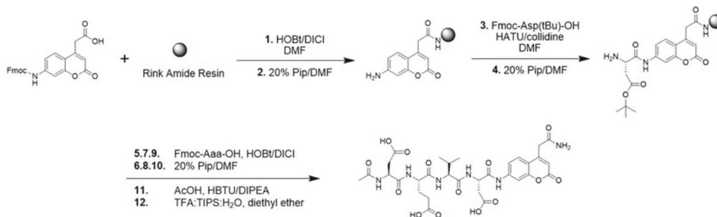
**Fig. 7** Scheme for synthesis of Ac-DEVD-ACC. The numbers from 1 to 12 indicate successive steps of the synthesis. (1) Fmoc-ACC-OH coupling to the resin; (2, 4, 6, 8, and 10) Fmoc group deprotection; (3) Coupling the first amino acid to the NH<sub>2</sub>-ACC-resin; (5, 7, and 9) peptide chain elongation; (11) acetylation of NH<sub>2</sub>-tetrapeptide-ACC; (12) substrate cleavage from the resin (removing protecting groups from the substrate) and substrate precipitation
