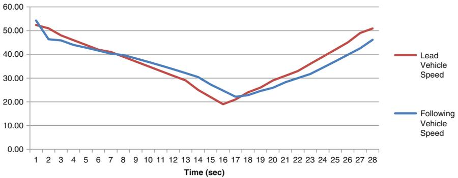
Fig. 2.4 Lead and following vehicle speeds for Example 2.1
