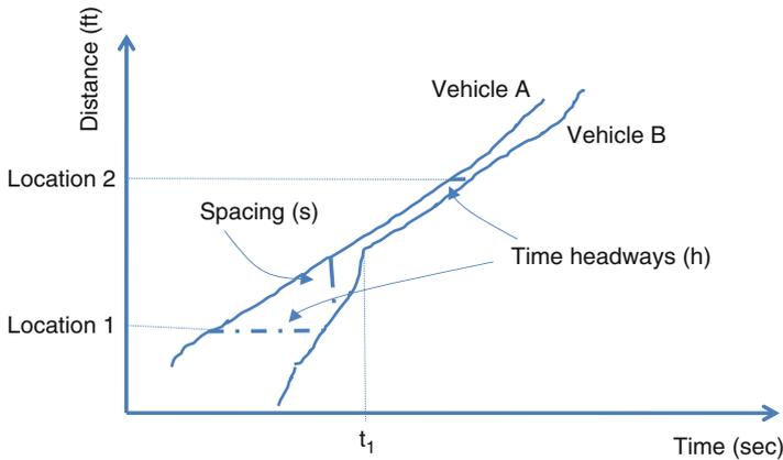
Fig. 2.1 Time-space diagram with two vehicle trajectories
