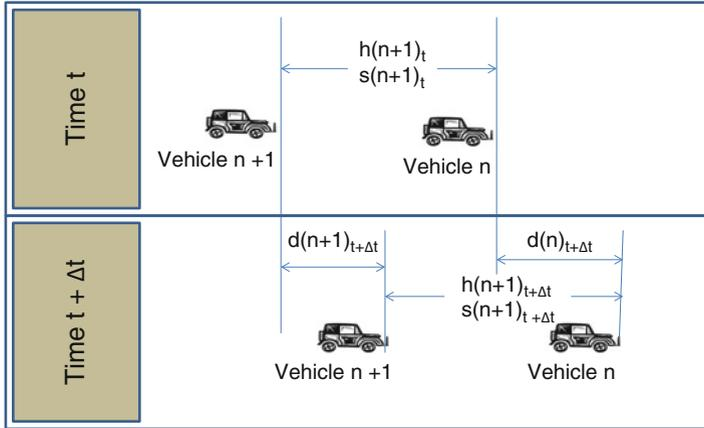
Fig. 2.3 Conceptual diagram and notation for car-following
