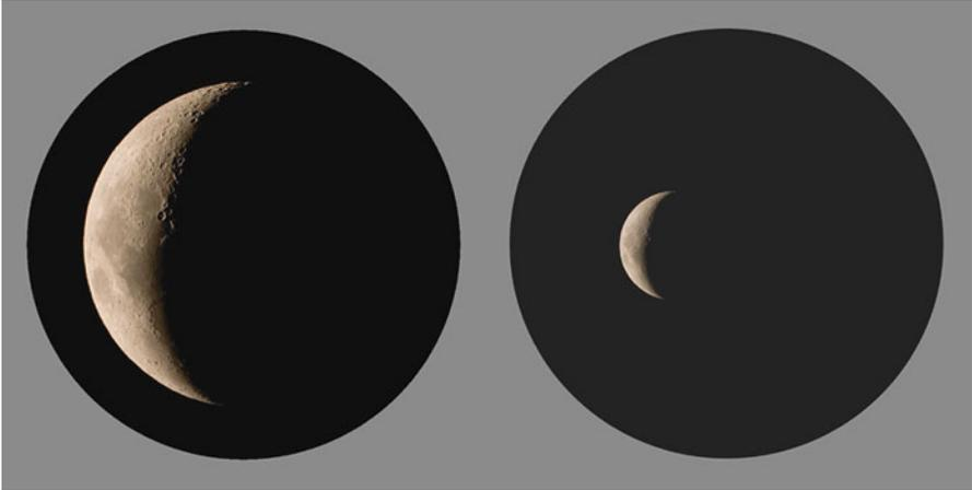
**Fig. 2.11** The Moon as it would appear in a 24 mm Panoptic eyepiece in a 203 mm (8 in.)  $f/10$  SCT (*left*) and with the same eyepiece in a 100 mm  $f/7.5$  refractor (*right*) (Moon astrograph courtesy of Mike Hankey, Freeland, MD, USA—[www.mikesastrophotos.com](http://www.mikesastrophotos.com))
