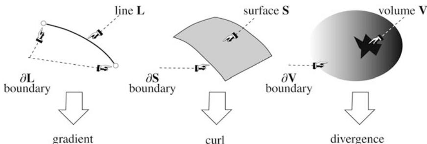
**Fig. 1.4** Topological notions at origin of three main differential operators
