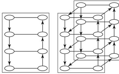
Fig. 1.3 Generation of space-time diagram from the space diagram
