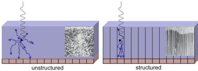
**Fig. 2.6** Schematic of an unstructured (*left*) and structured scintillator (*right*)
