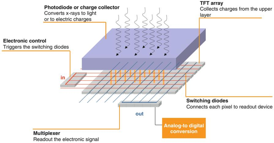
**Fig. 2.4** Flat-panel structure
