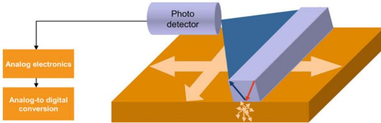
**Fig. 2.3** SPS scanning process; *SPS* storage-phosphor screens
