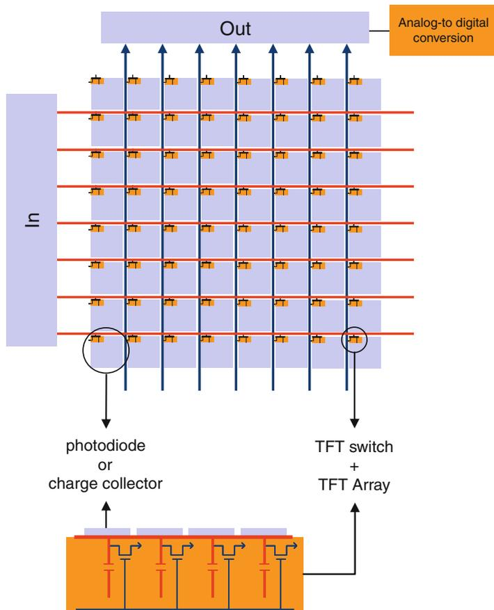
**Fig. 2.5** TFT array; *TFT* thin-film transistor
