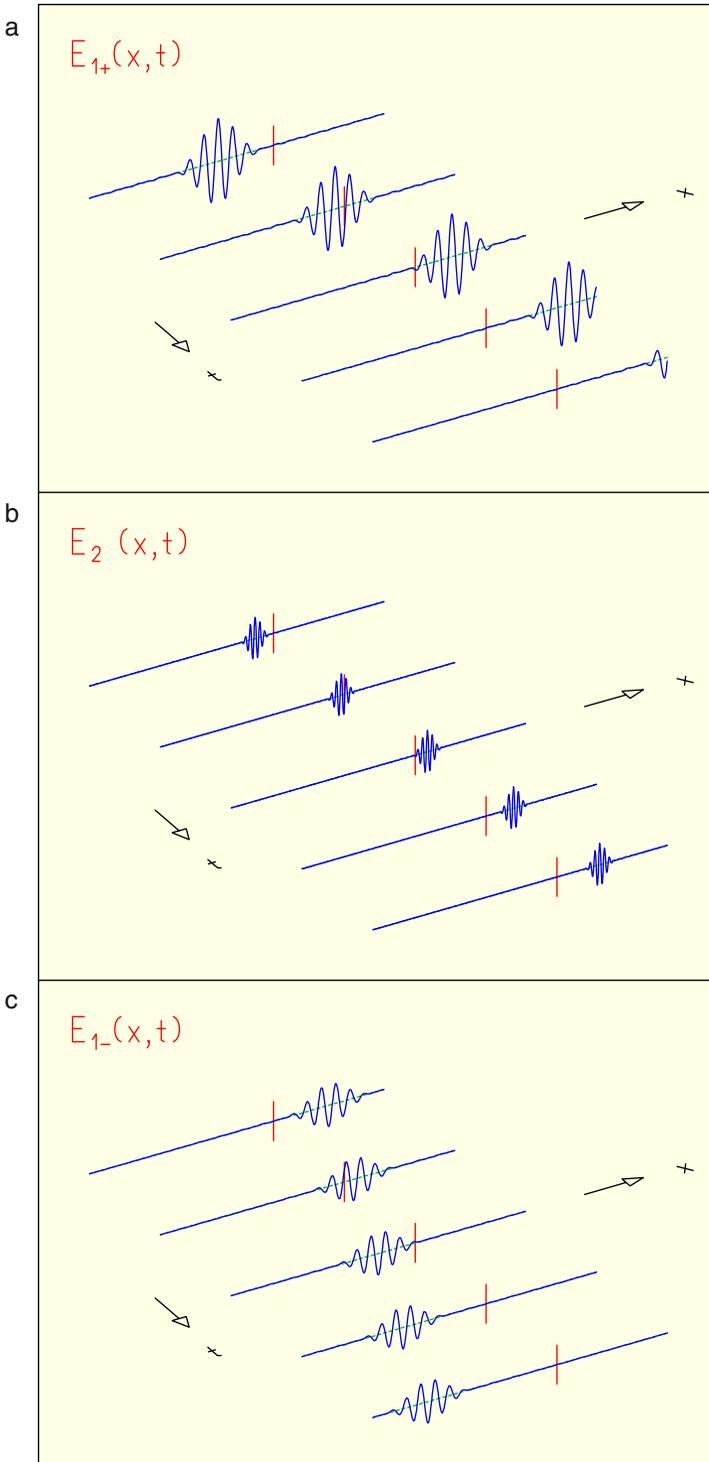
**Fig.2.11.** Time developments of the electric field strengths of the constituent waves in a wave packet of light incident on a glass surface: (a) incoming wave, (b) transmitted wave, and (c) reflected wave.
