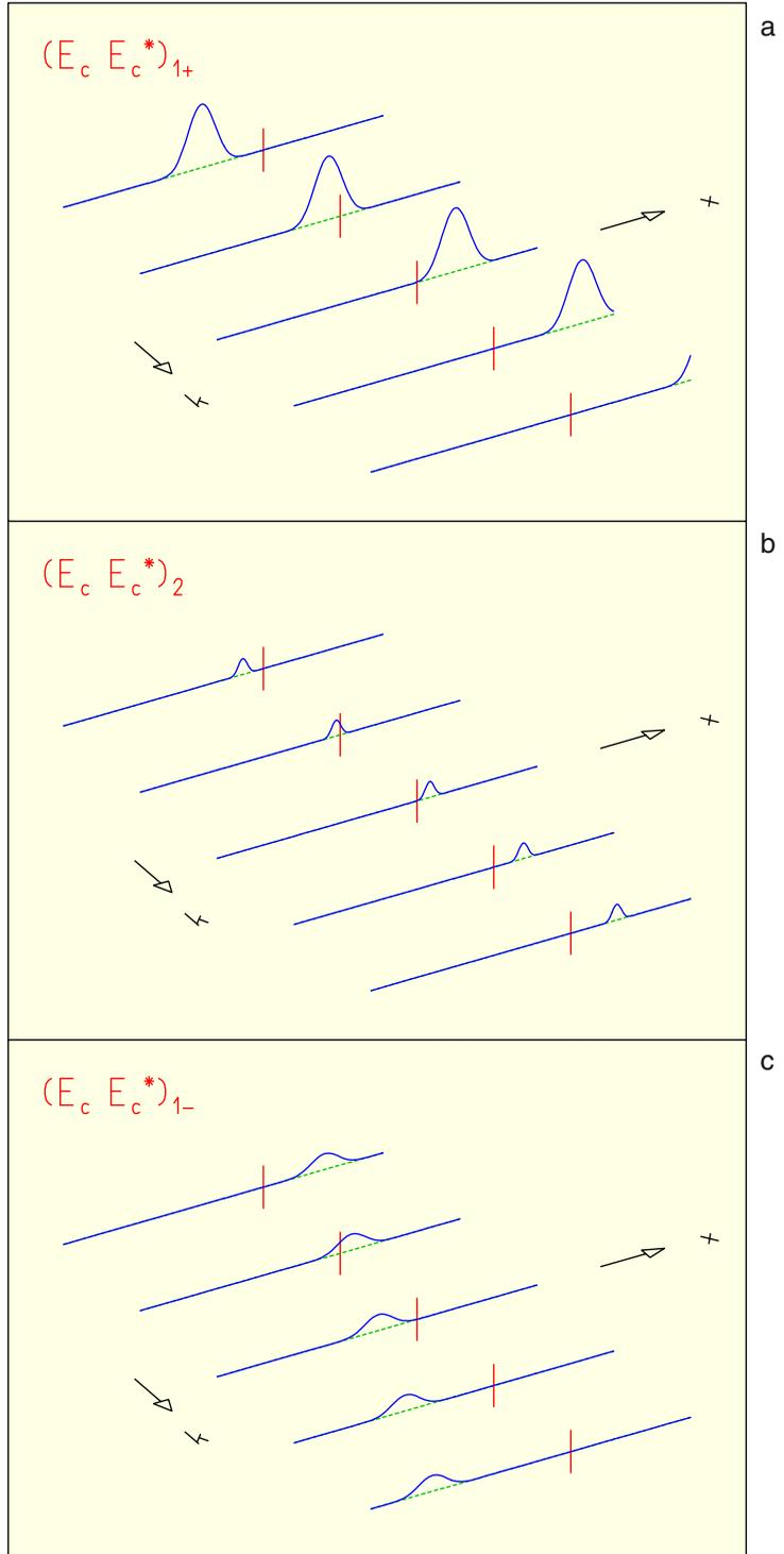
**Fig.2.10.** Time developments of the quantity  $E_c E_c^*$  (which except for a factor  $n^2$  is proportional to the average energy density) of the constituent waves in a wave packet of light incident on a glass surface: (a) incoming wave, (b) transmitted wave, and (c) reflected wave.
