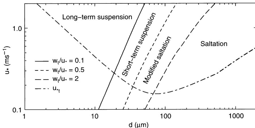
**Fig. 2.6** Threshold shear velocity and suspension modes for wind erosion of sand
