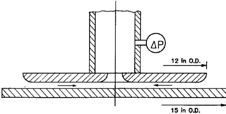
Fig. 2.7 Lift-off apparatus to determine the aerodynamic forces required to remove a dust deposit
