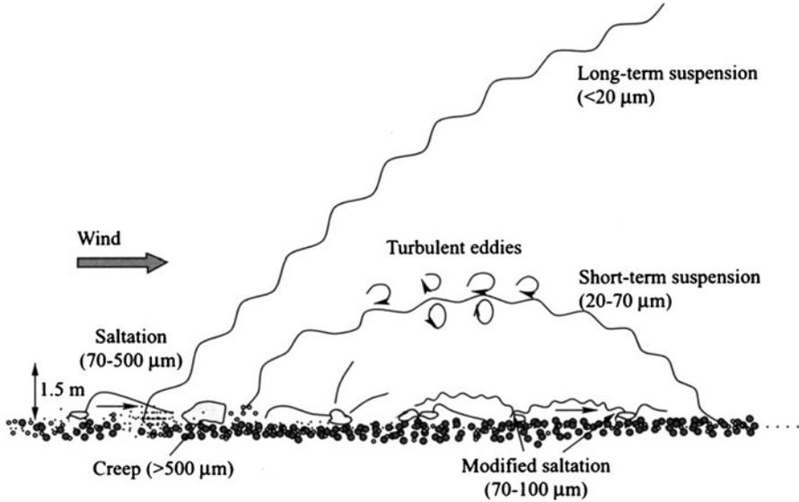
**Fig. 2.1** Different types of sand particle motion that can occur during wind erosion (from Shao, 2008)
