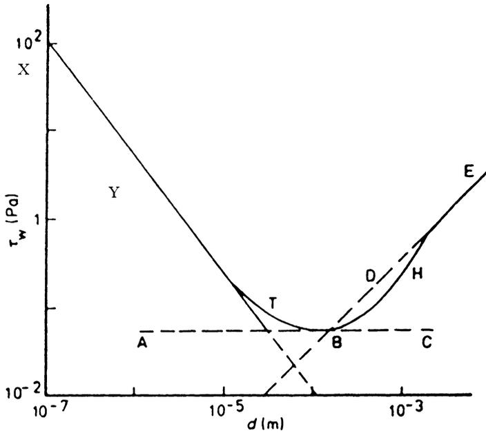
Fig. 2.5 Prediction of a force-balance theory for spherical sand particles in air
