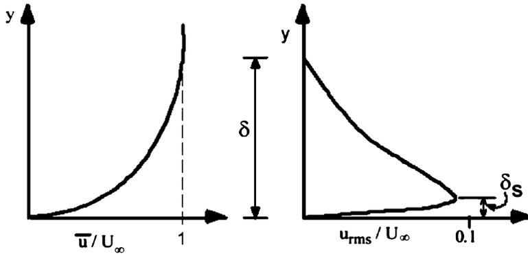
**Fig. 2.2** Typical streamwise velocity profiles inside the boundary layer: mean velocity (left), root mean square of the fluctuating velocity (right)
