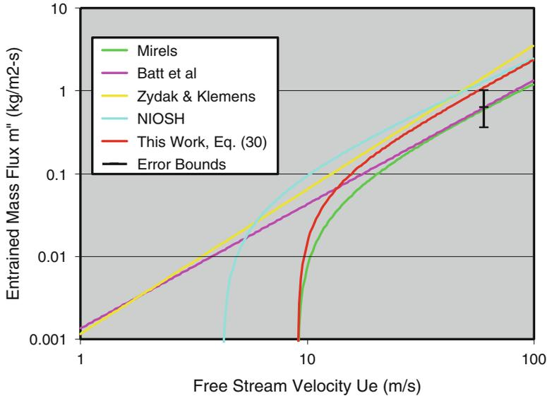
**Fig. 2.12** Comparison of the predictions from various entrainment mass flux equations for 53 micron coal dust
