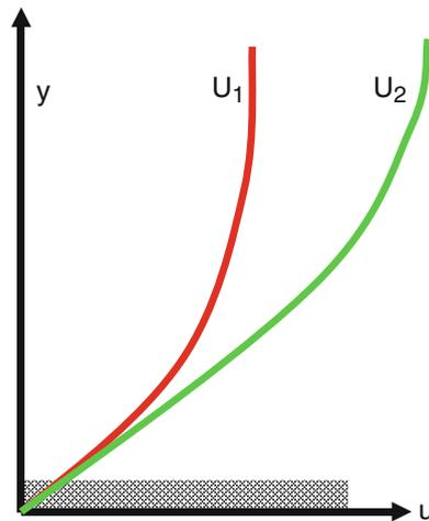
**Fig. 2.3** Typical streamwise mean velocity profiles inside the boundary layer for two different friction coefficients and free stream velocities
