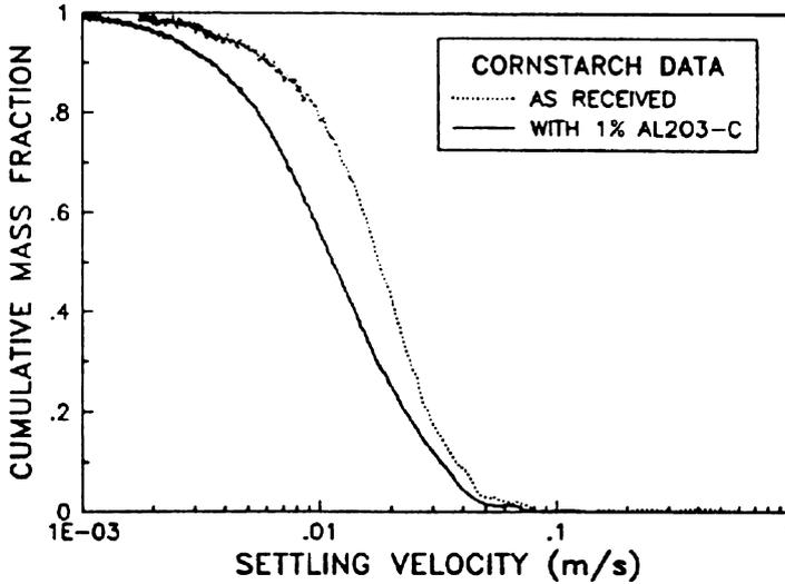
Fig. 2.4 Settling velocity of cornstarch with or without flowability agent Al<sub>2</sub>O<sub>3</sub>-C
