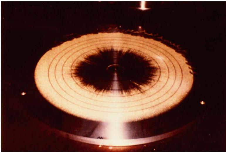
Fig. 2.8 Dust removal pattern in the lift-off apparatus
