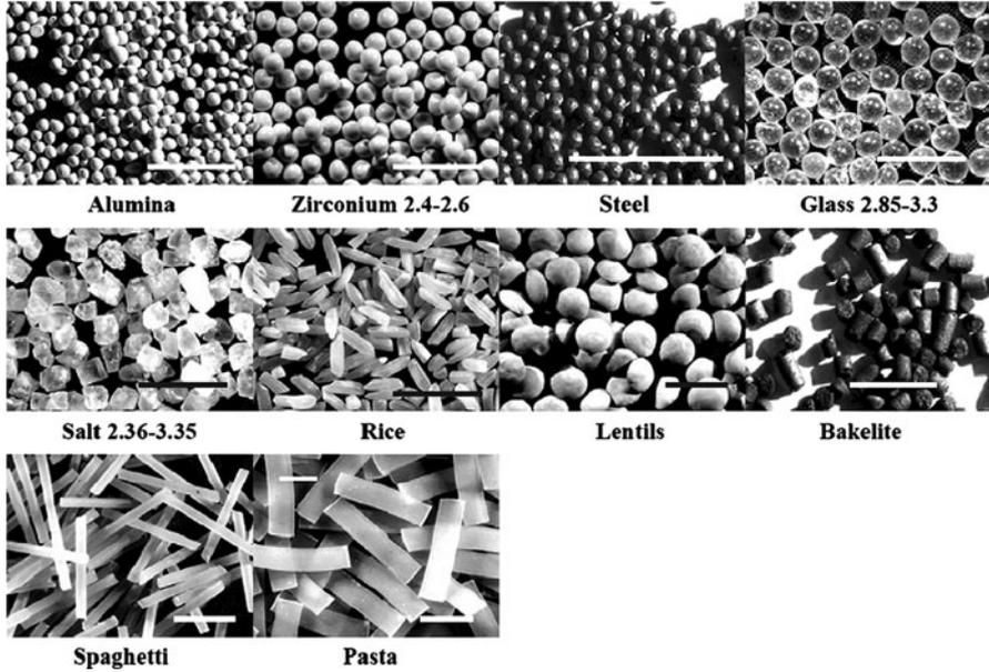
Fig. 2.10 Shapes of non-spherical particles
