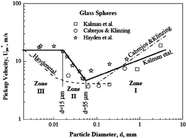
Fig. 2.11 Comparison of Kalman et al (2005) correlation with data for glass spheres and other correlations
