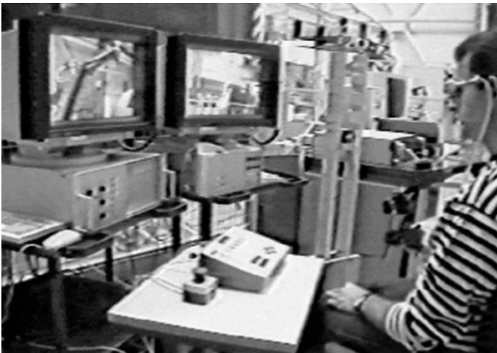
Fig. 2.5 The teleoperated robot is displayed simultaneously in real 3D images and using 3D artificial images
