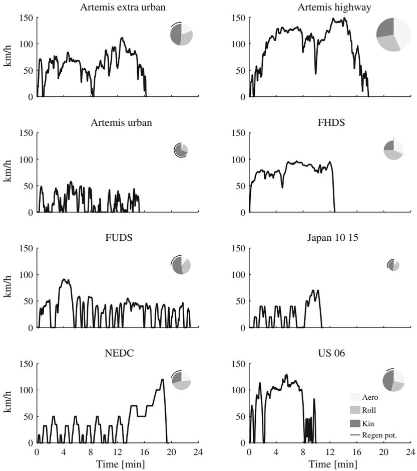
**Fig. 2.6** Some examples of standard driving cycles. The pie chart shows the relative amount of the energy terms  $E_{kin}^+$ ,  $E_{aero}^+$ ,  $E_{roll}^+$ , as well as the amount of kinetic energy that can be recovered according to (2.12). The pie surface is proportional to the total cycle energy  $E_{pwt}^+$  defined by (2.11). Energies are computed with the vehicle data of Table 8.1
