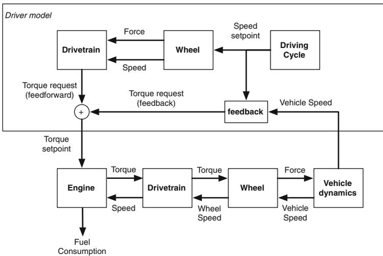
Fig. 2.4 Information flow in a backward–forward simulator
