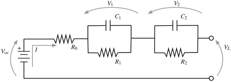
**Fig. 2.14** Battery equivalent circuit-based model (second-order)
