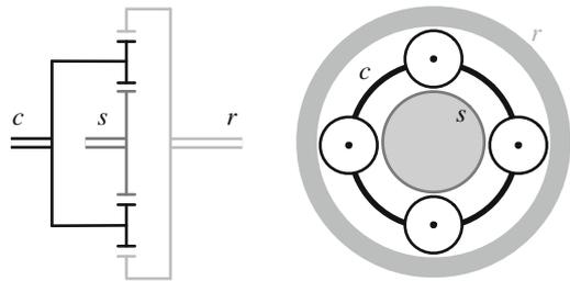
**Fig. 2.12** Torque balance on the planets
