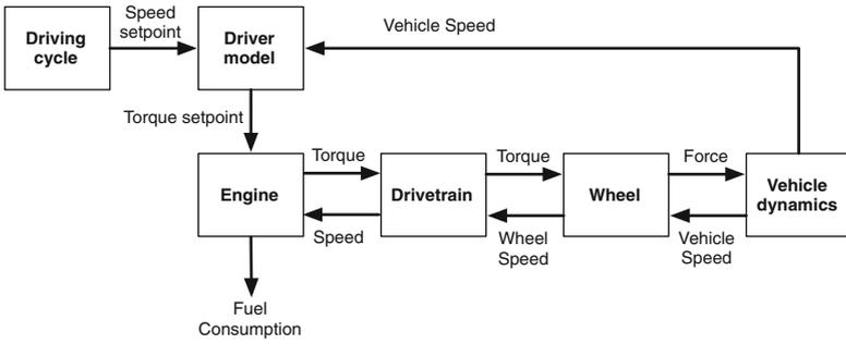
Fig. 2.2 Information flow in a forward simulator
