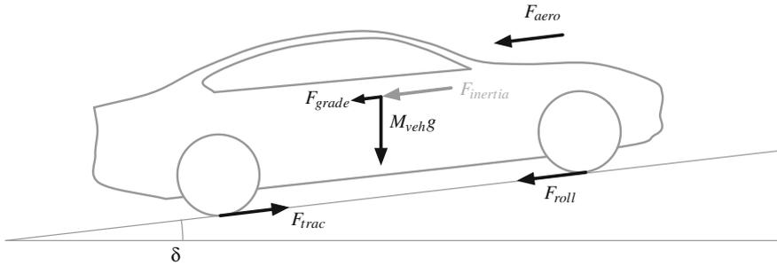
**Fig. 2.1** Forces acting on a vehicle
