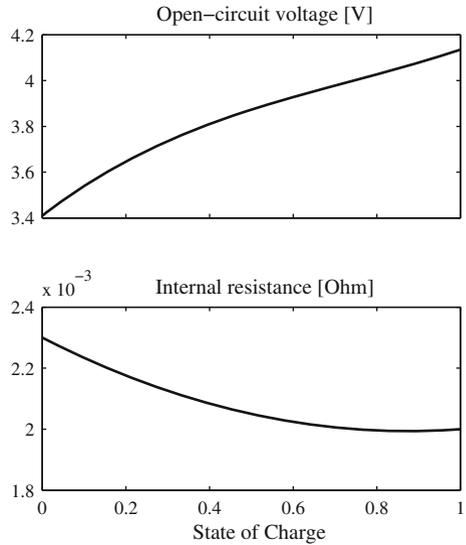
Apparently, integration of the current is sufficient to calculate the state of charge; however, in real-world applications, this is not stable (for numerical drift) nor accurate (for modeling approximations); therefore, more complex *SOC* estimation algorithms are used, which provide an estimate of the battery state of charge given available measurements of terminal voltage and current.
