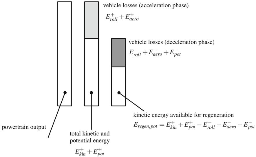
**Fig. 2.5** Vehicle energy balance (bar length represents energy)
