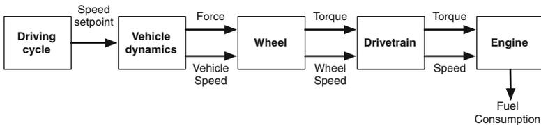
Fig. 2.3 Information flow in a backward simulator
