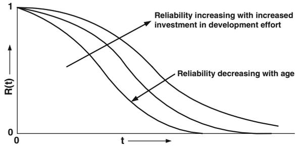
The reliability is given by a function  $R(t; \theta)$  with the following properties<sup>9</sup>:
