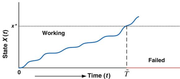
A typical example, where this characterisation is appropriate, is failure due to crack growth in a pipe. The state depends on the crack length, and failure occurs when the crack length reaches some critical value.
