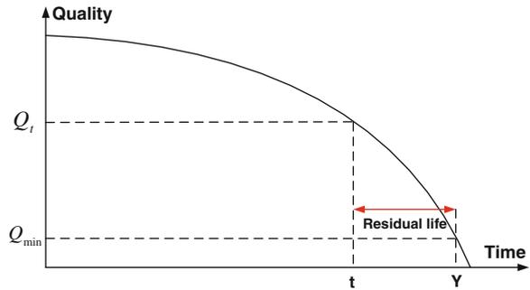
road. In Fig. 2.6 at time  $t$  (since the construction of the road), the quality is  $Q_t$  and  $Y$  denotes the time when the quality reaches the minimum acceptable level  $Q_{min}$  at which instant CM action is needed. The interval  $(Y - t)$  provides a window over which PM action can be initiated to avoid the need for CM action.
