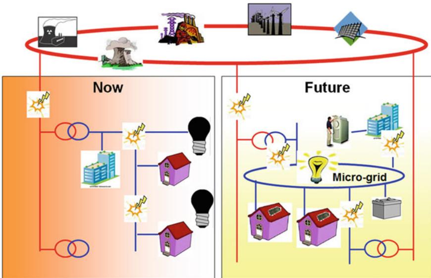
Fig. 4 Comparison of conventional grids with micro-grids
