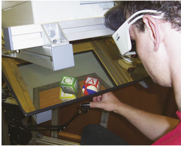
Fig. 2.14 Illustration of multi-point contacts using two Phantom 1.5 haptic interfaces
