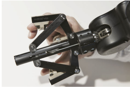
Fig. 2.1 Remote handling master hand interface mechanism. Courtesy of Oxford Technologies Ltd. ( www.oxfordtechnologies.co.uk )
