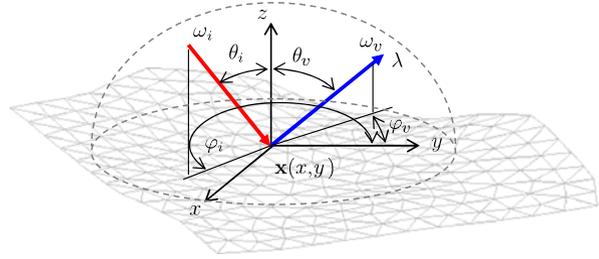
This model thus simultaneously represents both reflectance and transmittance properties of the GRF under the assumption that the incident light is partly reflected and partly transmitted from the incident location.
