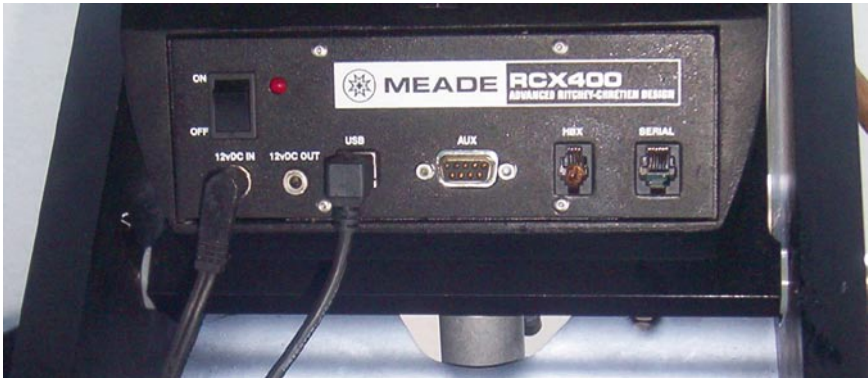
Fig. 2.5 Front panel of the LX400 telescope. Connectors left to right are for USB, auxiliary connection ( see text ), main handbox, and a serial connector
