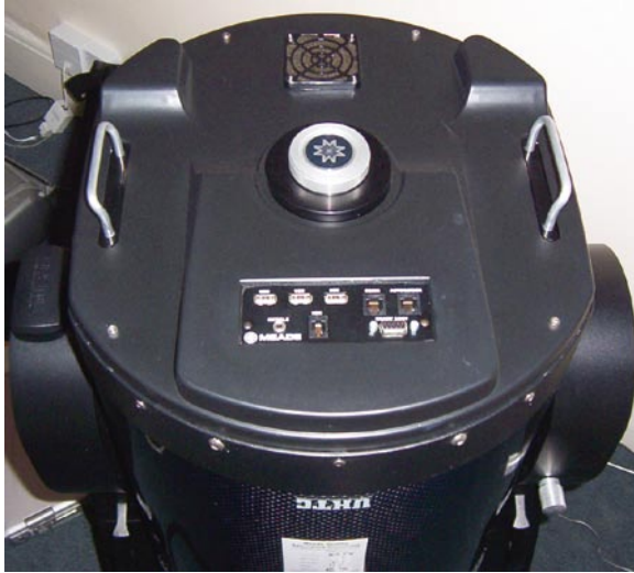
Fig. 2.6 Rear view of the LX400 showing handles, cooling fan, central visual back seal, and OTA connector panel
