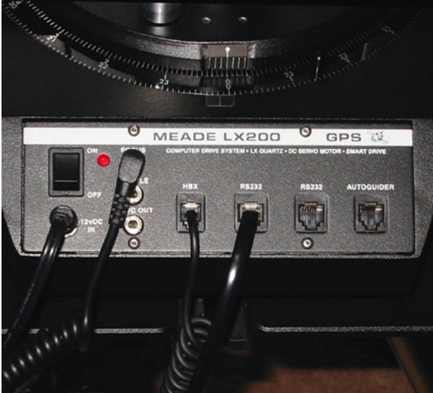
Fig. 2.4 Front panel of the LX200GPS telescope. The electronic focuser connection is to the right of the power connection; other connectors ( left to right ) are for the handbox, serial connectors (RS232), and the autoguider port
