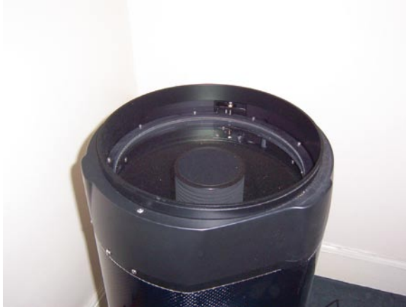
Fig. 2.2 The front end of the 30-cm LX400 showing the corrector plate. Focusing is achieved by motors driving the corrector plate within the OTA
