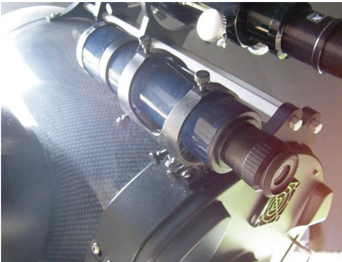
Fig. 2.7 Meade LX200GPS/LX400 Finder mounted on an LX400. The guide scope can be seen above it. It is important to align the finder on a bright target object visible in the main scope. This allows easy guidescope use
