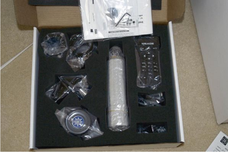
Fig. 2.3 LX400ACF accessories box as first opened. The package includes the handbox, finderscope, right-angled prism, cables, and assorted adapters. A picture can be very helpful should you need to repack for transport
