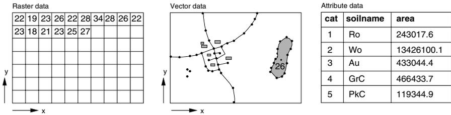
**Fig. 2.1.** Data models in GIS – raster and vector data with attribute table:
