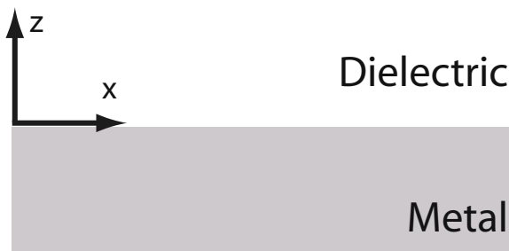
Figure 2.2. Geometry for SPP propagation at a single interface between a metal and a dielectric.
