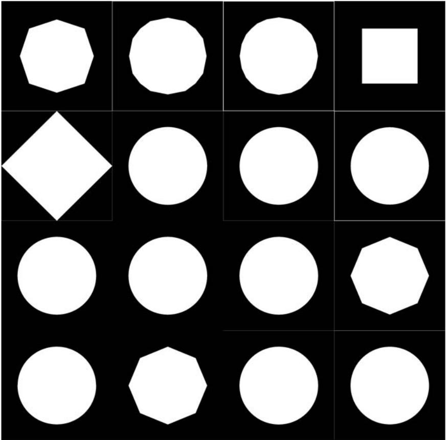
**Figure 7.** Thresholded results of various distance transform algorithms applied to an image consisting of a solitary object consisting of a single point at the center of the image. Top row, left to right: CDA 3x3, CDA 5x5, CDA 7x7, Chessboard. Second row, left to right: Cityblock, CSED, DRA 3x3, DRA 7x7. Third row, left to right: DV, 8SED, 8SED modified, Euclidean 3x3. Fourth row, left to right: 4SED, MD, MDDR, SimpleList.
