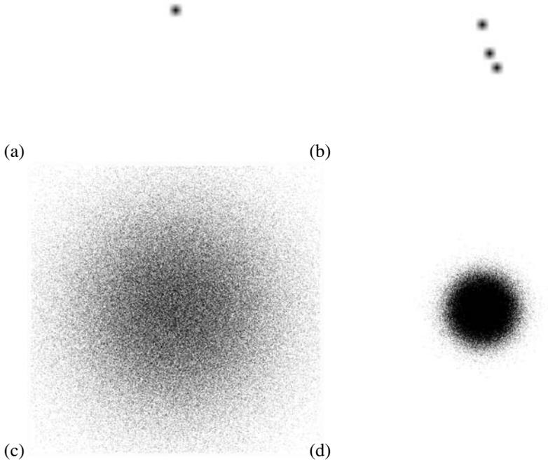
**Figure 2.** Sample test images consisting of (a) a single, solitary point-object, (b) a configuration of three single point-objects that is a known problematic configuration, (c) and (d) randomly generated test images by sampling from a normal distribution (with different standard deviations).
