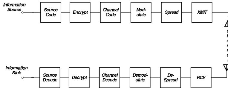
**Fig. 0.1.** Block diagram of modern digital communications system
