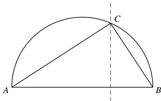
Figure 2.17: Constructing a right-angled triangle with given hypotenuse
