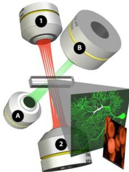
**Fig. 7.** BioPhotonics Workstation: Information Optics drives the creation of purposely patterned light can perform assorted functions, such as enabling higher microscope resolutions, initiating spatially controlled light-driven biochemical processes, and exerting finely calibrated forces, while leaving enough room for integrating other auxiliary systems. (adapted from [24])
