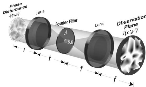
**Fig. 1.** Generic common path interferometer based on a  $4f$  optical system. The diffraction orders representing spatial frequency components of an input phase disturbance, obtained at the back-focal plane of a Fourier transforming lens, are filtered to phase-shift selected components to be used to synthesize a reference wave. Subsequent recombination at the observation plane generates an interference pattern. (adapted from [6], © OSA 2007)
