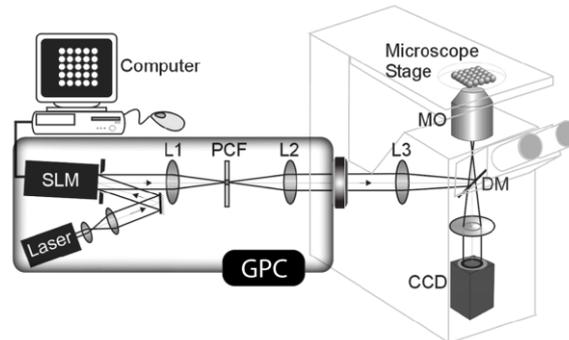
**Fig. 5.** Optical trapping and manipulation. Light patterns synthesized by a GPC illumination module are relayed to a microscope as optical traps for manipulating microparticles. (adapted from [17], © OSA 2002 )
