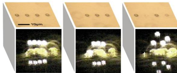
**Fig. 6.** Interactive microscopy using GPC-generated beams for controlled manipulation of multiple particles. Top: Optical setup with GPC-generated light patterns creating multiple counter-propagating beam traps. Another microscope is fitted orthogonally for enhanced observation. Bottom: Composite of top- and side-view microscope images obtained from the system. (adapted from [18], © OSA 2005)
