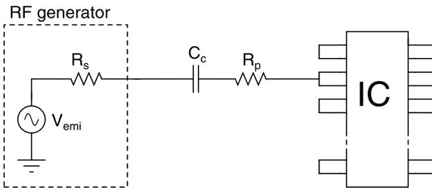
Figure 2.8. Direct power injection measurement setup.
