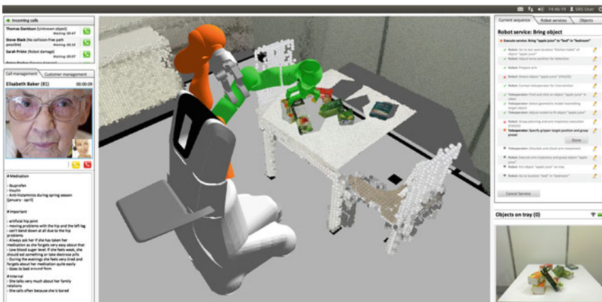
Fig. 7 User interface for professional teleoperators
