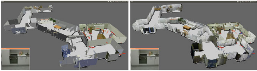
Fig. 8 User interface for professional teleoperators with central area maximized and in zoomed-out perspective. Left Environment visualization with geometric 3D mapping. Right Environment visualization with voxel-based 3D mapping
