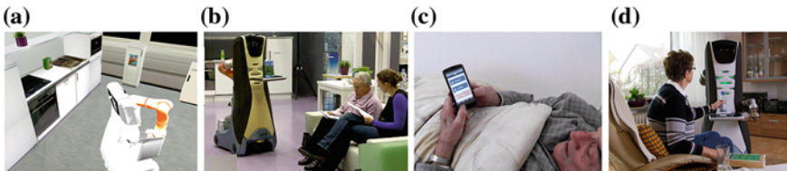
Fig. 4 Evaluation of the user interface for elderly people. a Lab evaluation where robot simulation showed robot actions in modeled home environment. b Evaluation in model kitchen. c and d Evaluation in real homes of elderly people
