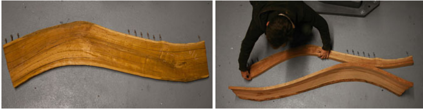
Fig. 7 Left sample flitch, with nested cuts and dowel holes. Right in-progress assembly
