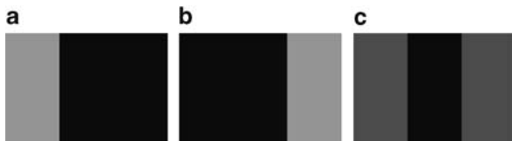
Fig. 2.10 Three different 3 \times 2 images consisting of vertical lines: a f_1 ; b f_2 ; c I_3 . Here, black denotes a grey-scale value of zero, light grey a grey-scale value of 4, and the darker grey a grey-scale value of 2
