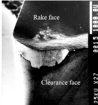
Figure 2.13. Example of flank wear for CVD diamond tool in machining MMC ( V_c = 50 m/min, f=0.2 mm/rev, d_{oc}=1 mm and cutting time 4.5 min) [14]
