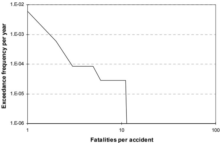
**Figure 2.9.** f-N curve for offshore installations, all fatalities
