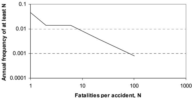
Figure 2.1. Example  $f$ - $N$  diagram
