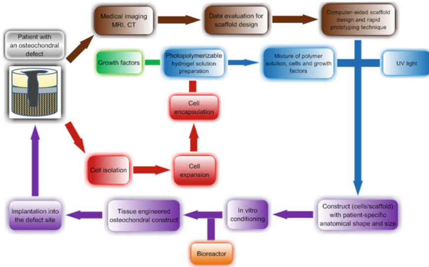
Fig. 2.6 Step-wise strategy for the patient-specific treatment of an OC defect. The data obtained from medical imaging, such as magnetic resonance imaging (MRI) or computed tomography (CT) is used in the design of a scaffold that is specific for the patient. Autologous cells are isolated and expanded in vitro and encapsulated into the photopolymerizable polymer solution where also growth factors are introduced. Then, the construct (cell/scaffold) is manufactured with a rapid prototyping technique under UV light to obtain the anatomical correct shape and size. The cellular scaffold is dynamically conditioned in vitro with a bioreactor. The tissue engineered OC construct is then implanted into the OC defect of the patient
