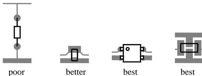
Figure 17-12. Connecting Signal and Ground to a Transient/Surge Protector
