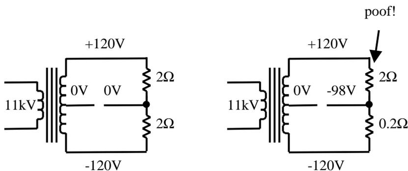
Figure 17-2. AC Surge Voltage from Open Neutral Conductor
