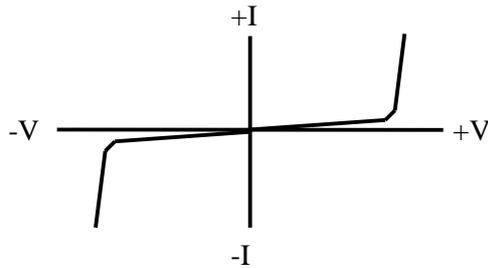
Figure 17-7. Typical V-I Curve for a Bidirectional Clamp
