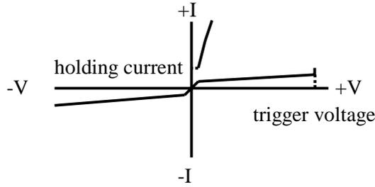
Figure 17-9. Typical V-I Curve for a Unidirectional Crowbar
