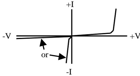
Figure 17-6. Typical V-I Curve for a Unidirectional Clamp
