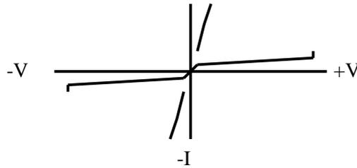
Figure 17-10. Typical V-I Curve for a Bidirectional Crowbar
