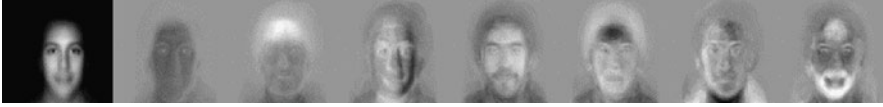
Fig. 2.2 Eigenfaces: the average face on the left, followed by seven top eigenfaces. From Turk and Pentland [36], with permission
