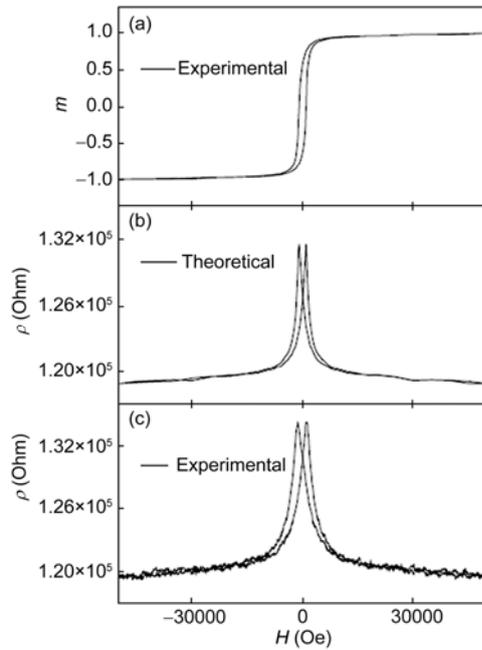
**Figure 7** Direct comparison among the experimental  $m$ - $H$  curve (a), the theoretical  $\rho$ - $H$  curve by spin dependent variable range hopping model (b), and the experimental  $\rho$ - $H$  curve (c) measured at 5 K for the  $\text{Ti}_{0.24}\text{Co}_{0.76}\text{O}_2$  magnetic semiconductor film. Copyright 2006 IOP Publishing Ltd, reproduced from ref. [110] with permission.
