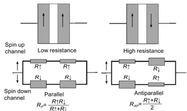
**Figure 5** Schematic of the resistor model for GMR. For the parallel state (left panel), the spin-up channel is the majority spin channel in both the ferromagnetic layers, experiencing a low resistance. For the antiparallel state (right panel), each spin channel has been strongly scattered in one of the ferromagnetic layers, showing a high resistance. Copyright 2008 IOP Publishing Ltd, reproduced from ref. [39] with permission.
