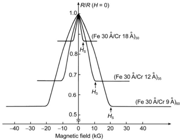
**Figure 2** Original measurement of the GMR by the group of Albert Fert in three Fe/Cr magnetic superlattices at 4.2 K. During the measurements, both the current and the applied field were applied in the film plane and were parallel to the [1 1 0] axis. Copyright 1988 American Physical Society, reproduced from ref. [2] with permission.
