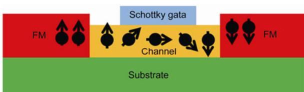
Figure 6 Schematic of the proposed Datta-Das spin-FET [88].
