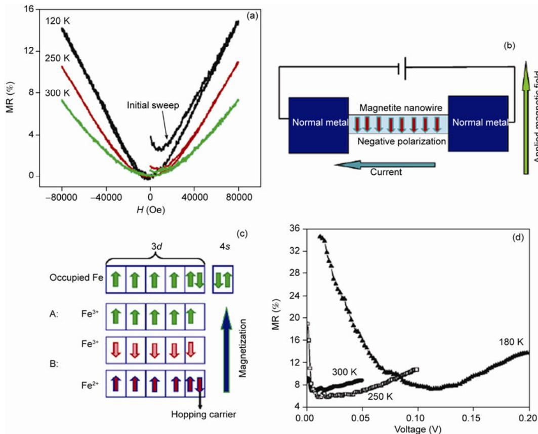
**Figure 8** (a) MR of individual  $\text{Fe}_3\text{O}_4$  nanowires measured at different temperatures. (b) Schematic of the device. (c) FM order of  $\text{Fe}_3\text{O}_4$ , where the minority carriers are responsible for the transport. (d) Bias dependence of MR for the  $\text{Fe}_3\text{O}_4$  nanowire-based devices. Copyright 2006 American Chemical Society, reproduced from ref. [117] with permission.
