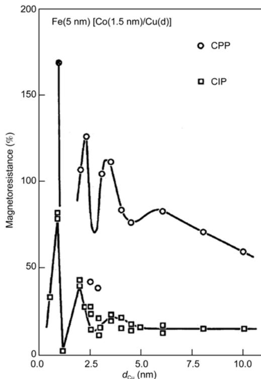
**Figure 4** Nonmagnetic Cu space layer thickness dependence of both the CPP and CIP GMR. Copyright 2002 Elsevier Science B.V., reproduced from ref. [35] with permission.
