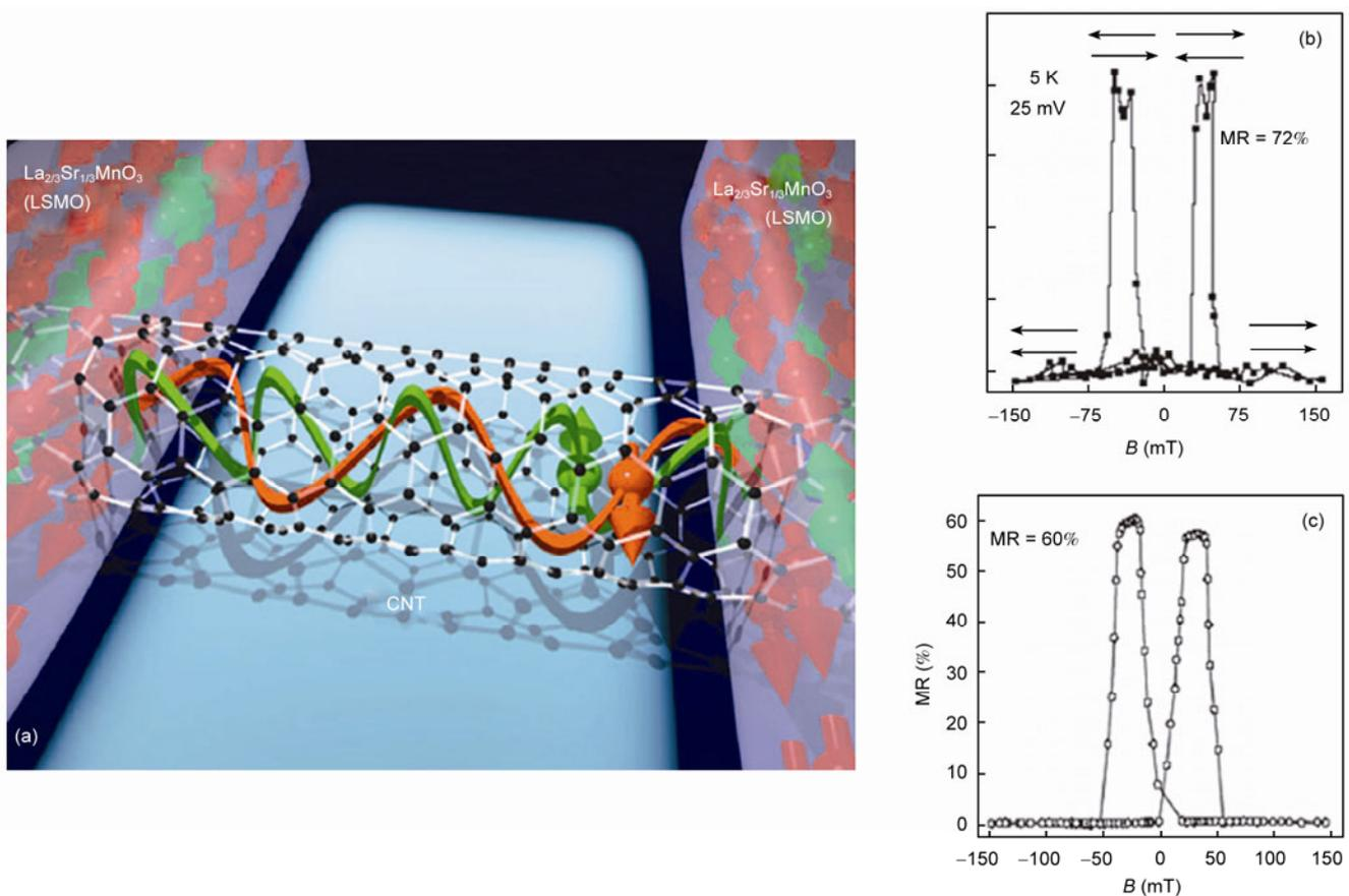
**Figure 9** (a) Artistic view of spin transport through a carbon nanotube (CNT) between magnetic (LSMO) electrodes. (b) and (c) are the low temperature experimental data. A contrast of 72% and 60% is obtained between the resistances for the parallel (high field) and antiparallel peaks magnetic configurations of the source and drain. Copyright 2008 American Physical Society, reproduced from ref. [124] with permission.
