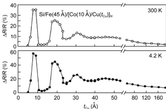
**Figure 3** Dependence of the saturation MR on the Cu interlayer thickness for Si/Fe(45 Å)/[Co(10 Å)/Cu( $t_{Cu}$ ) $_N$ ] superlattices.  $N=16$  for  $t_{Cu}$  below 55 Å and  $N=8$  for  $t_{Cu}$  above 55 Å. Copyright 1991 American Physical Society, reproduced from ref. [13] with permission.
